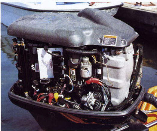
Above: The computerised high-pressure direct injection system makes the Mercury Optimax 150 Dig two-stroke more fuel-efficient than an equivalent-sized four-stroke. Right: "The combination of boat and engine was well-matched. I didn't need any tricks to get it going."
