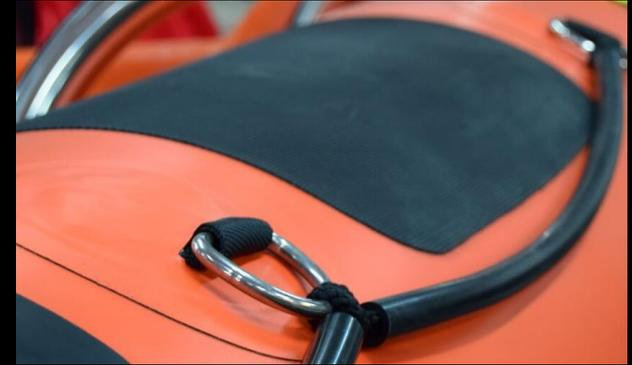
External Life lines mounted on 'D' ring safety line holders
