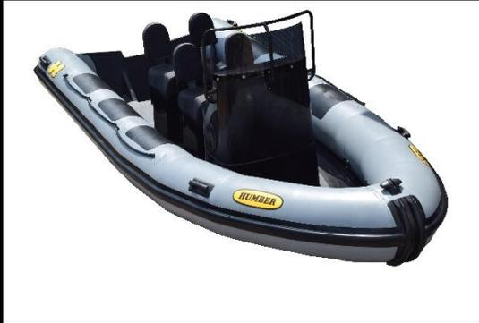
Mini double 'D' outer tube rubbing strake
