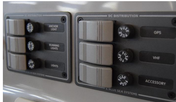
Switch panel, fused waterproof with twin bus bars (Required for electric items)
