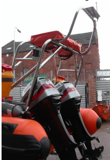
Self-Righting frame (Aluminium) with inflation bag, cylinder, valise & fitting head
