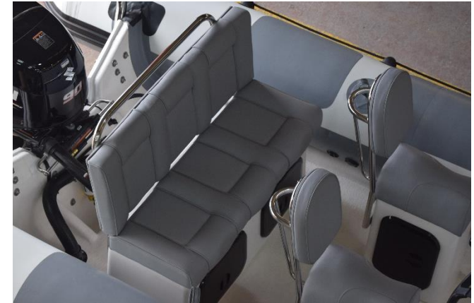
Bench seat, two person with fixed back rest & twin storage compartments
