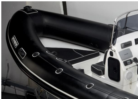
Bow cushion with side tube mounted grab loops
