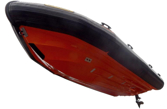
Lifting points, heavy duty - 4 off Suitable for crane lifting *Excludes lifting strop
