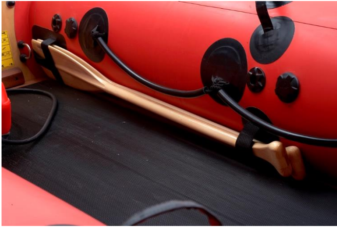
Life lines, internally mounted on rear straights of tubes, 2 loops each side
